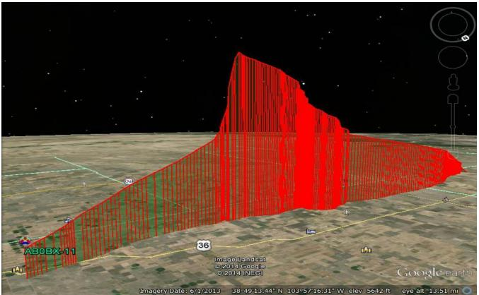
Flight Path Looking Southwest, max altitude was about 102,800 feet. Launch is small 'tail' at extreme-right, final beacon is on left when it was still above 10,000'. The faster the balloon was moving horizontally, the farther apart the beacon lines. It traveled at speeds of about 4mph to about 50mph.
